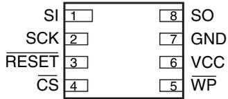
Figure 2-2. SOIC Top View
